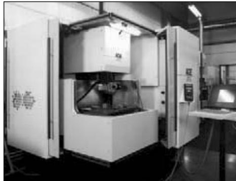
Wire erosion EDM machine
